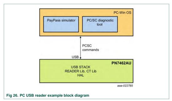
The USB stack and CCID class is implemented in the PN7462AU. The default CCID driver present in PC with Windows OS is used for operation.
