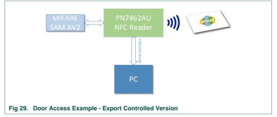
On power-up, NFC Reader starts polling for (PICC) cards (Type A, B or F, ISO15693, ISO18000-3M3) and if no card is present, the reader goes to standby mode. Timer is used as a wakeup source from standby - timer periodically every 500 ms. This process continues until a card is detected by the RF field of the reader. If a card is detected, the card type with its UID is sent via HSU & this is printed on the PC console
