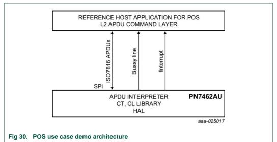
The POS demo architecture is split into application layer (L2) and low level EMVCo compliant layer L1 which is hosted on the PN7462AU. The application layer L2 commands are simulated in reference microcontroller board (LPC1769) and L1 layer components are placed in PN7462AU.
