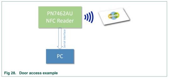
After each polling loop the application goes to standby mode and remains for 500ms. A timer is used as a wakeup source from standby. This process continues until a card is detected by the RF field of the reader. If a card is detected, the card type with its UID is sent via HSU and will be printed on the PC console.
