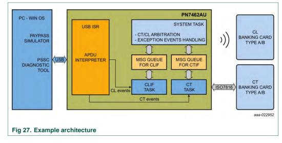
Note: Detailed description and how to use example is described in "PN7462AU PC CCID Reader User Manual".
