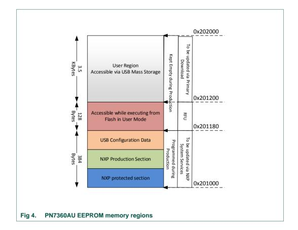
Note: The RFU section of 128 bytes is kept hidden from the aperture of USB mass storage. But this area is used by the HAL executing from the user flash for internal purposes. As of now, there is no special use case for this region and hence in the default examples of PN7462AU, this region remains unused.
