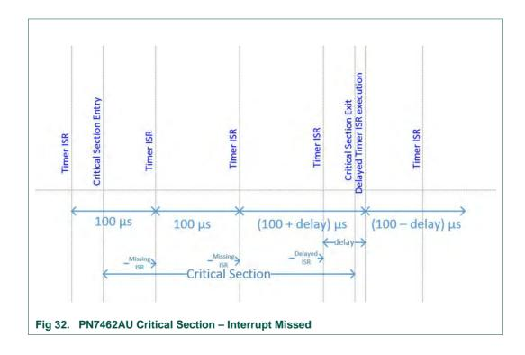
As presented in the Fig 32 there is a possibility of missing interrupts when the interrupt is configured to occur every 100 µs and if the interrupt arrives when the "*phhalRf\_Receive()*" API is executing the critical section in passive target mode, the interrupt gets missed couple of times.
