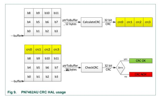
• Check the CRC of a buffer of arbitrary length with supplied CRC. The supplied CRC shall be last 2 bytes or 4 bytes of the buffer.
